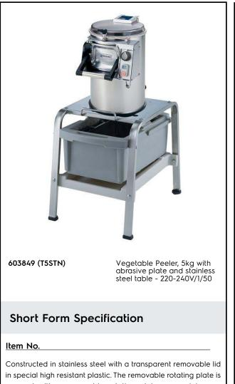
covered with a removable rotating plate covered in very resistant abrasive material (silicon carbide). An interlocking safety magnetic devices will stop the machine from operating when the lid or door is opened. The electronic controls and motor have IP55 protection. Simple control panel with ON/OFF buttons and timer. Supplied with an abrasive plate and stainless steel filter table
